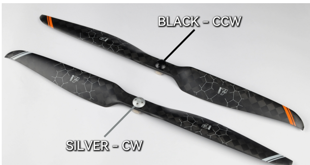
Step 1: Distinguishing between CCW and CW Propellers
