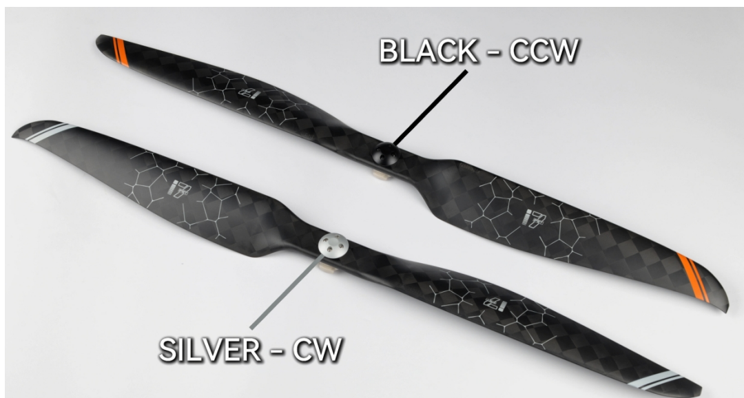
Step 1: Distinguishing between CCW and CW Propellers
